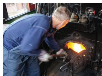
▲ The fireman stokes the firebox in Locomotive 136 with coal.
